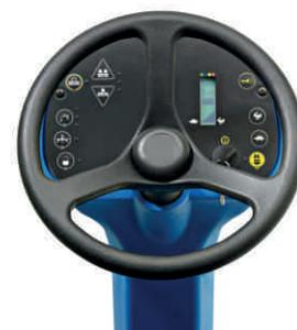
One Touch scrubbing button is conveniently located on the easy-to-understand control panel.
